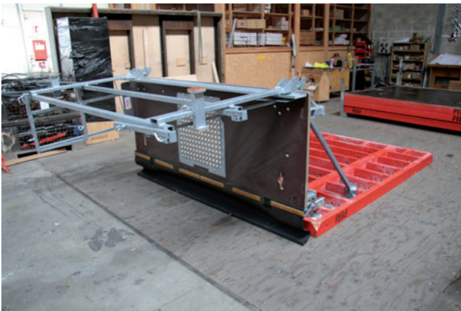
5. Secure diagonal bracing in the panel struts.
